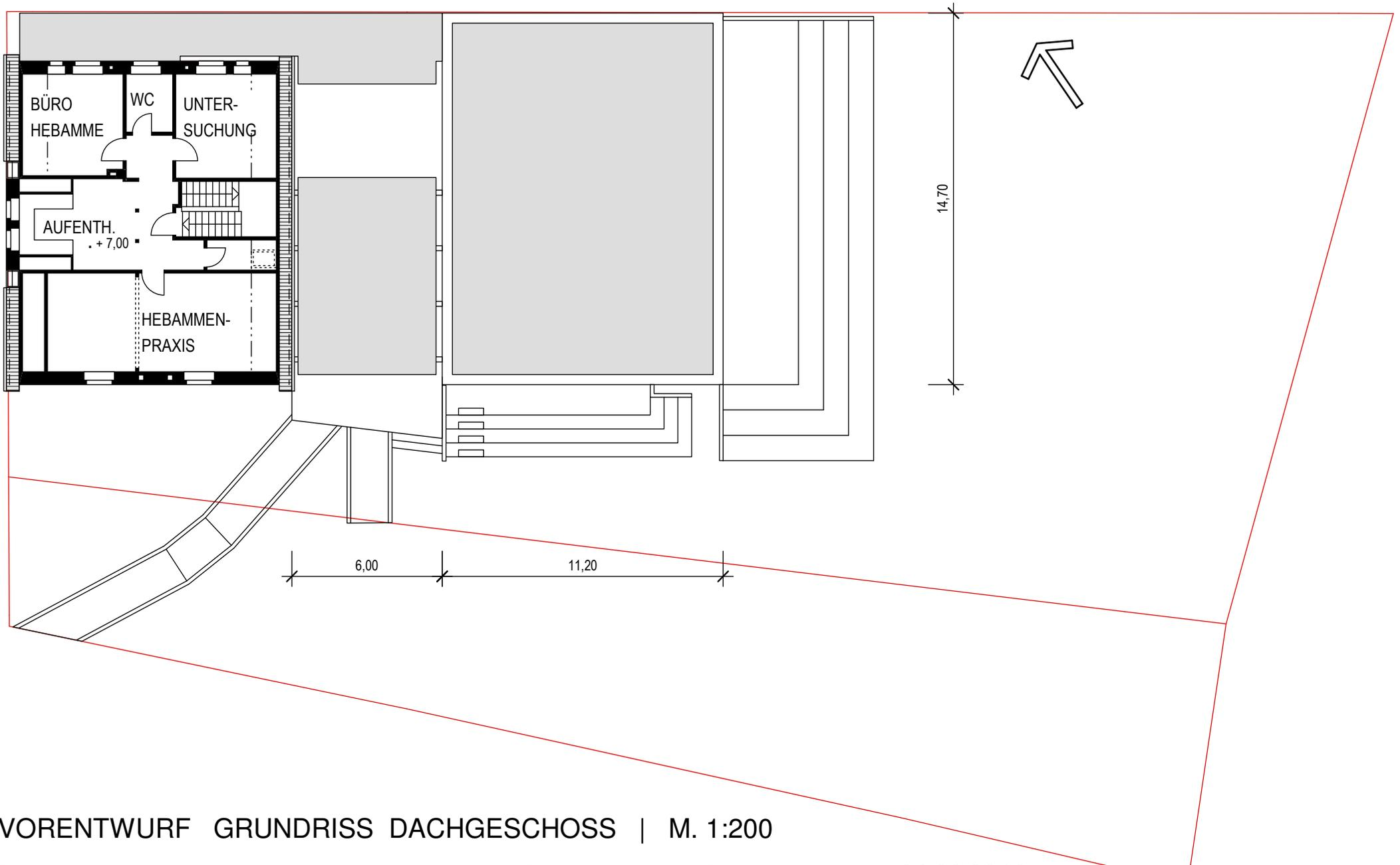
VORENTWURF GRUNDRISS DACHGESCHOSS | M. 1:200
